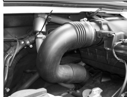
Figure 5 Remote Mounted SER, Convenient Access for Cleaning.
